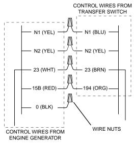
Figure 1. Wire Connections
